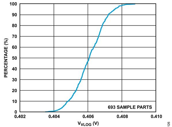
Figure 26.  $V_{VLOG}$  at  $I_{INP} = 1 \text{ nA}$  Distribution
