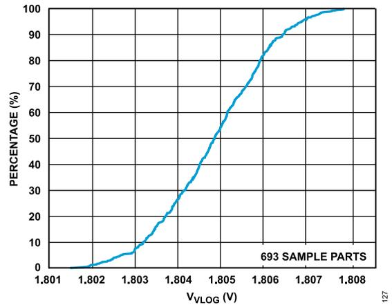
Figure 27.  $V_{VLOG}$  at  $I_{INP} = 10 \text{ nA}$  Distribution
