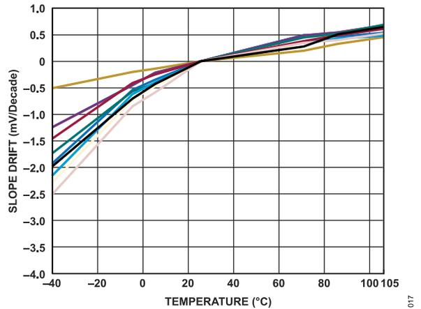
Figure 14. Slope Drift vs. Temperature Over 10 Samples
