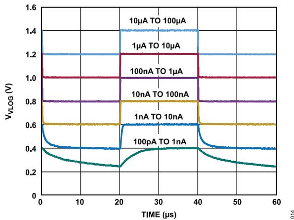
Figure 24. Pulse Response for  $I_{INP}$  in Decade Steps
