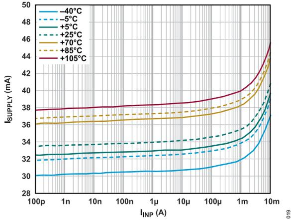
Figure 16. Supply Current vs.  $I_{INP}$  at Various Temperatures
