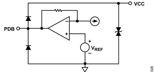
Figure 37. Simplified Schematic of PDB Interface
