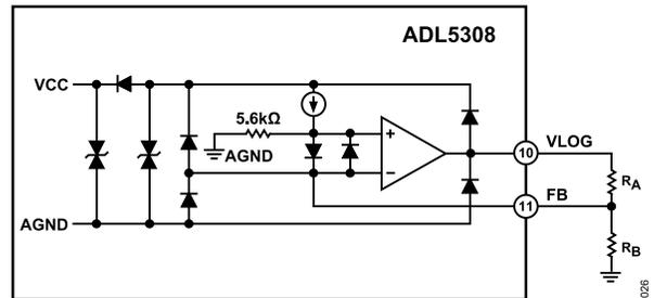
Figure 33. Simplified Schematic of VLOG and FB Interface
