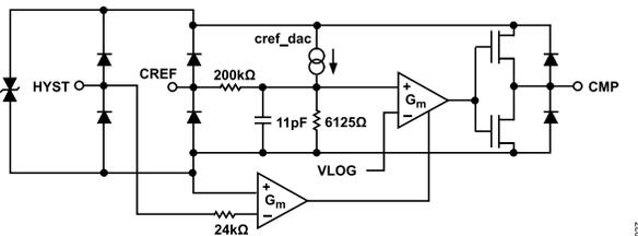
Figure 36. Simplified Comparator Interface for  $CREF\_DAC > 0$
