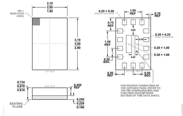
Figure 42. 14-Terminal Land Grid Array [LGA] (CC-14-4)
