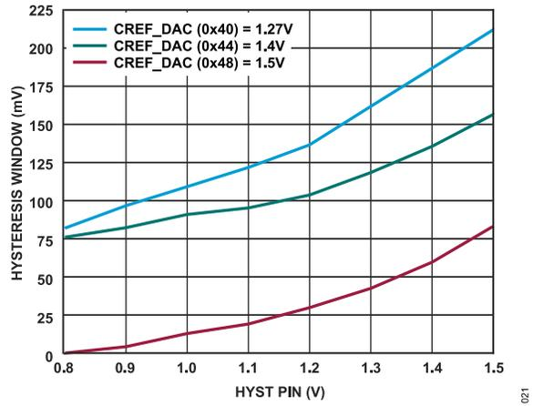
Figure 29. Calculated Comparator Hysteresis at Various  $CREF\_DAC$  Value
