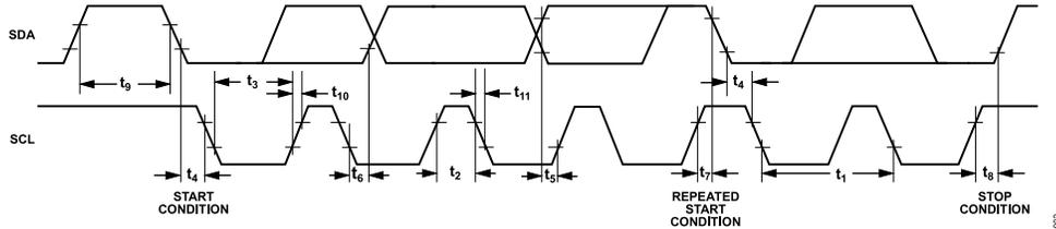
**Figure 2. I<sup>2</sup>C Timing Diagram**
