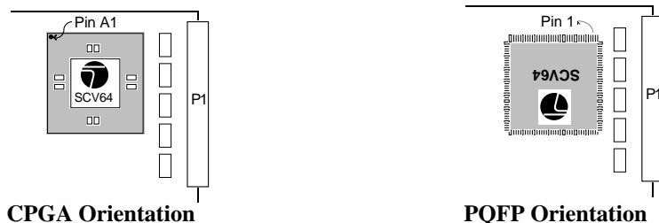
Figure E.1 : Orientation of the SCV64 (CPGA and PQFP) to Minimize Distance to the Connector
