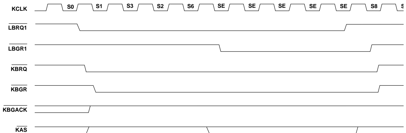
Figure 2.19 : Local Arbitration for External Device - Without Acknowledgment
