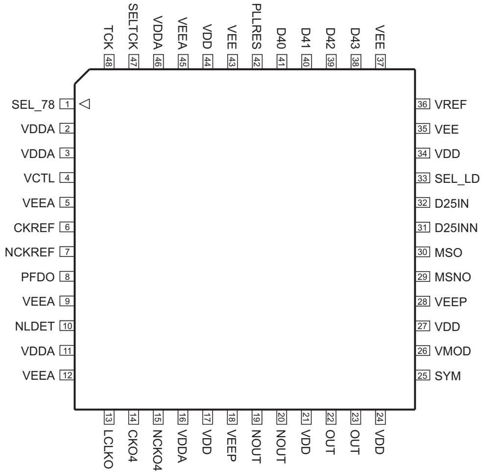
Figure 6. Package Pinout, 48 Lead TQFP - Top View
