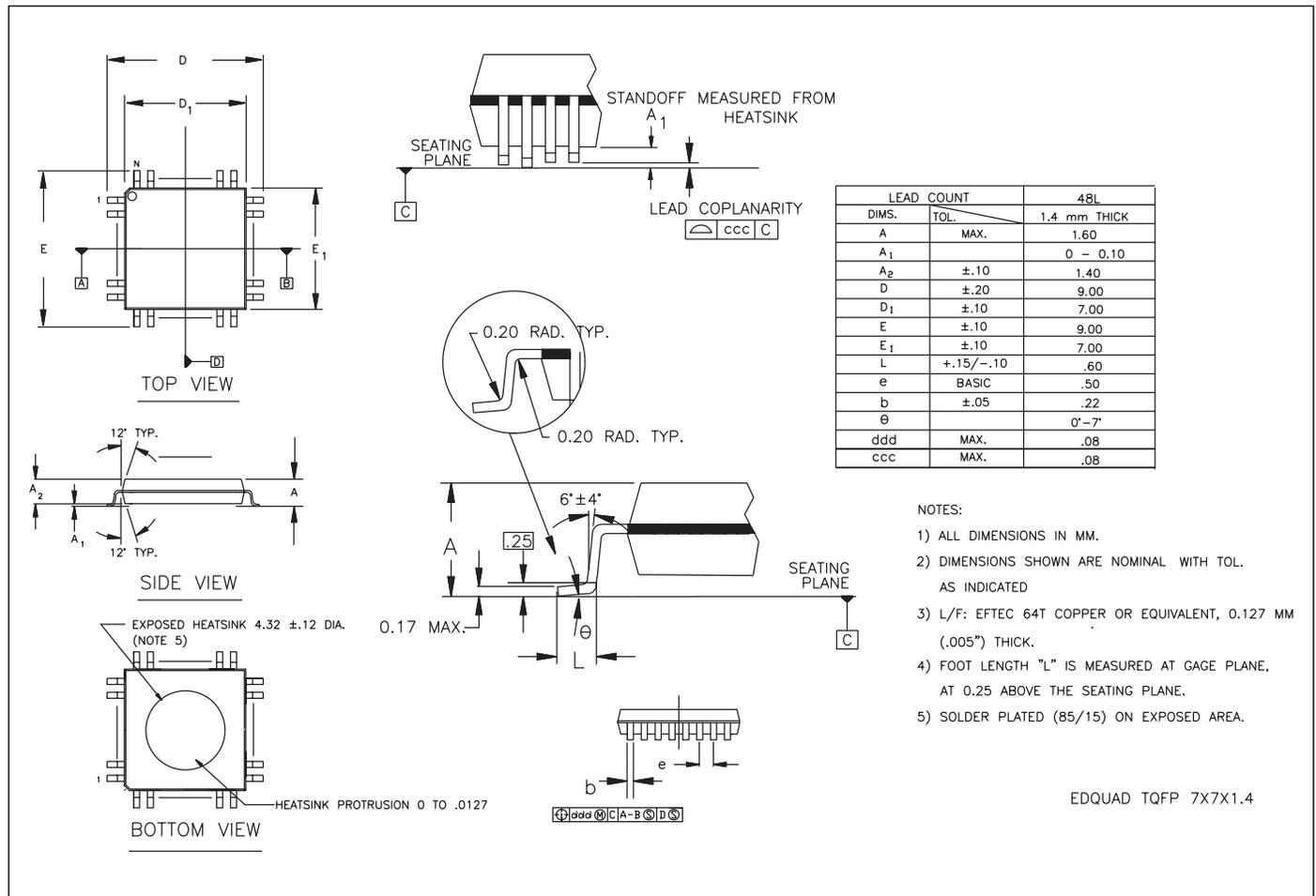
Figure 7. Package 48 Lead TQFP, Power Enhanced
