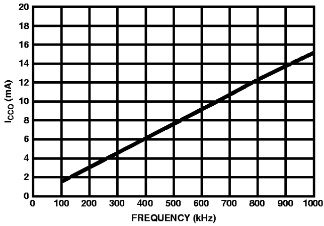
FIGURE 2. I_{CCO} vs FREQUENCY
