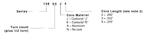
In this example, the 138 series was ordered with 4 1/2 turns, and a carbonyl "J" core with a length of .375".
