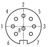
Contact arrangement (Plug-in side)
