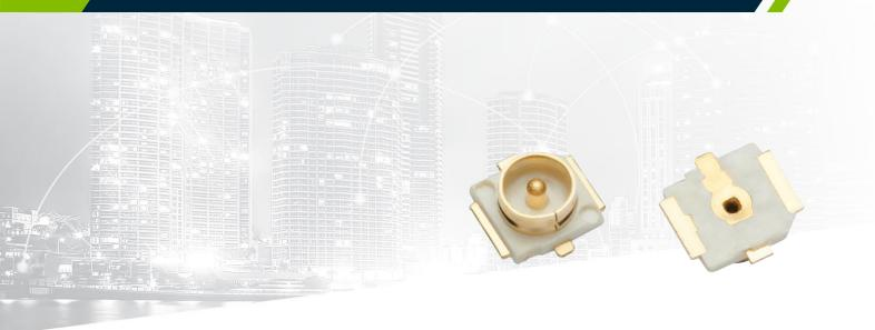
Part of the Taoglas SMD Mount Receptacle, the RECE.20279.001E.01 is a 3-pad type wire-to-board SMD receptacle that is ultra-small, lightweight and low profile, 2.5mm max. With an operational frequency range of DC to 6 GHz the RECE.20279.001E.01 is gold plated to provide superior performance and allow for ease of mounting with the male RF connector.
