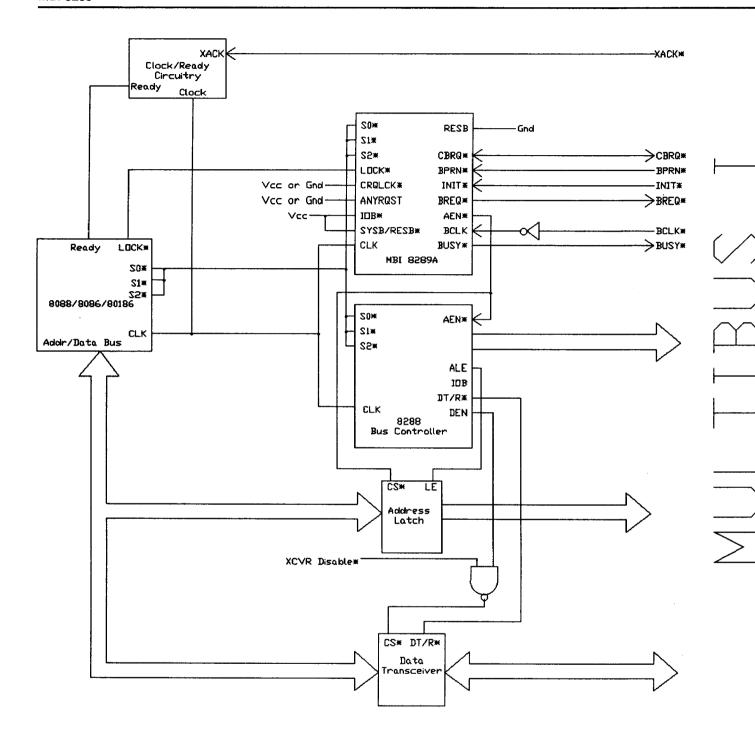
Figure 2. MBI 8289A System Configuration (Single Bus System)
