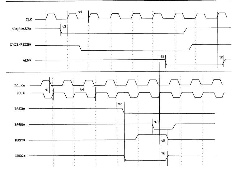
Figure 3. MBI 8289 Timing Diagram
