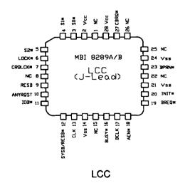
Figure 1. Pinout of MBI 8289
