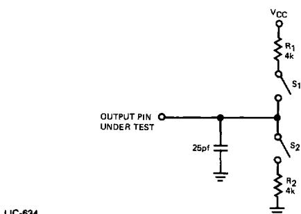
Test Circuit for DBIN to 8080A BUS
