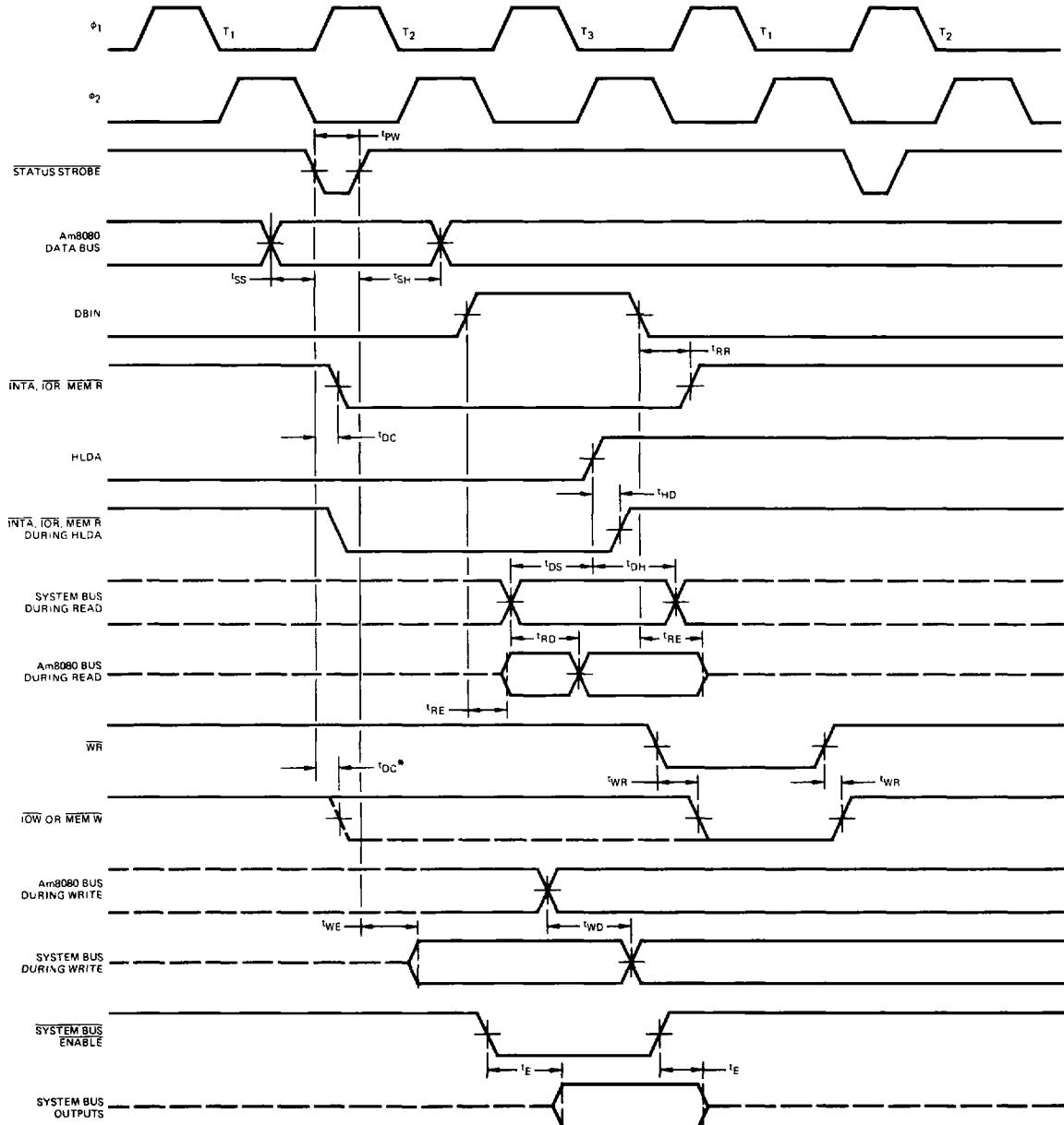
Voltage measurements points:  $D_0 - D_7$  (when outputs) Logic "0" = 0.8 V, Logic "1" = 3.0 V. All other signals measured at 1.5 V.
