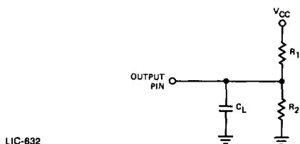
Note 1. For D<sub>0</sub>–D<sub>7</sub>: R<sub>1</sub> = 4.0 kΩ, R<sub>2</sub> = ∞Ω, C<sub>L</sub> = 25 pF.
