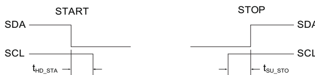
Figure 2: I 2 C STOP and START Conditions; START: A High "1" to Low "0" Transition on the SDA Line While SCL is High "1" STOP: A Low "0" to High "1" Transition on the SDA Line While SCL is High "1".
