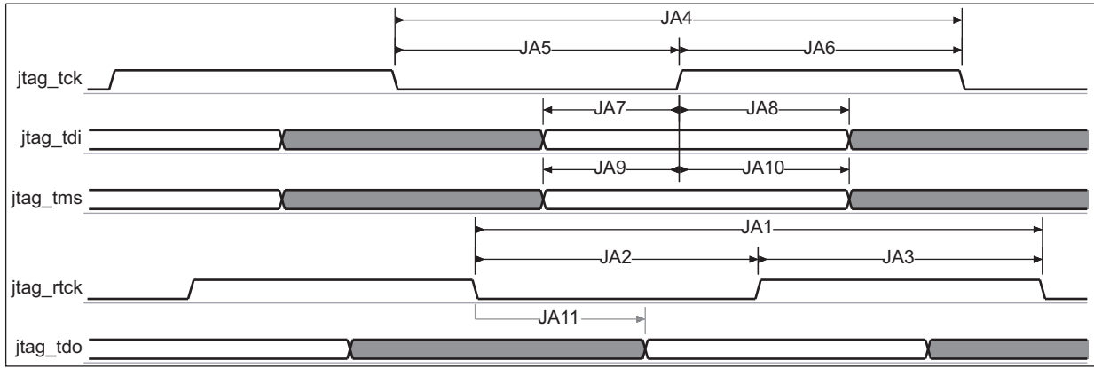
Figure 6-67. JTAG Interface Timing – Adaptive Clock Mode
