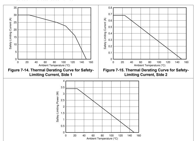
Figure 7-16. Thermal Derating Curve for Safety-Limiting Power
