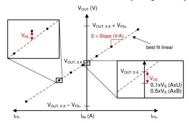
Figure 8-1. Sensitivity, Offset, and Nonlinearity Error
