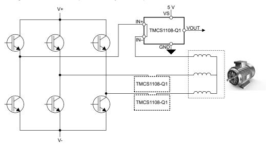
Figure 10-2. Inline Motor Phase Current Sensing
