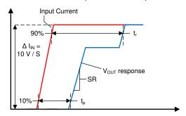
Figure 8-4. Current Overload Transient Response
