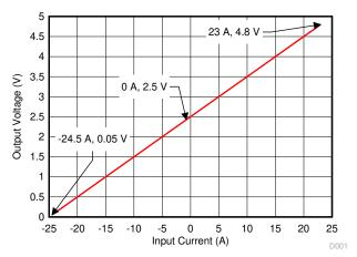
Figure 10-3. Application Example Design Transfer Curve
