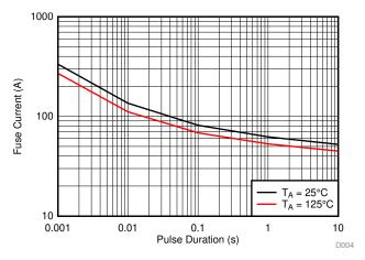
Figure 8-10. Single-Pulse Leadframe Capability
