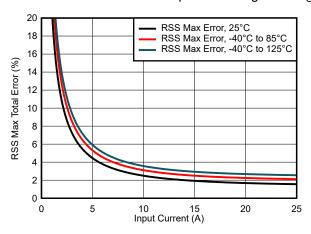
Figure 10-1. RSS Error vs Input Current
