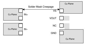
Figure 12-2. Layout for System Creepage Requirements
