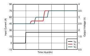
Figure 8-2. Transient Step Response
