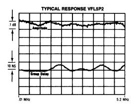
We have designed many Lowpass Filters for the video field having sharp roll-offs and good passband delay linearity with cut-off frequencies from .1 MHz to 10 MHz. The most popular of these are used to attenuate the harmonics of the NTSC color sub-carrier frequency 3.58 MHz. The most commonly used filters in this group are tabulated below:
