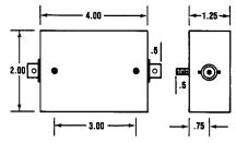
VFL series with B.N.C. connectors size =  $4'' \times 2'' \times 114''$ VCL series with B.N.C. connectors size =  $5'' \times 2'' \times 114''$
