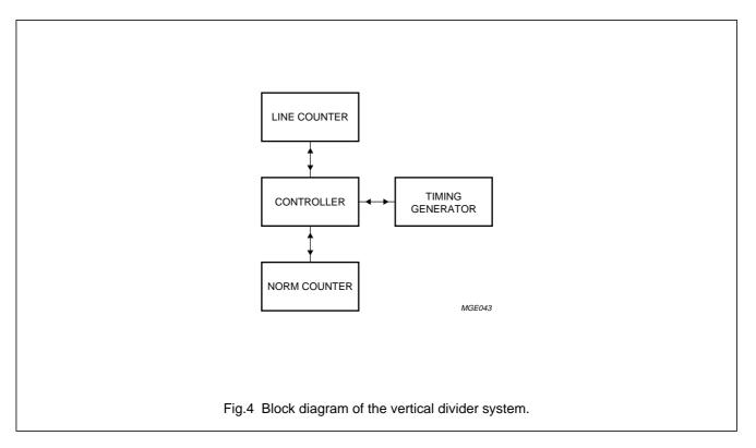
The divider system operates at twice the horizontal frequency. The line counter receives enable pulses at this frequency, thereby counting two pulses per line. A state diagram of the controller is shown in Fig.5. Because it is symmetrical only the right-hand part will be described.
