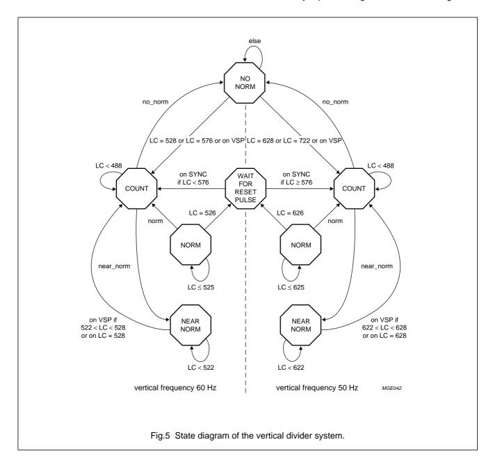
When the controller is in the NEAR\_NORM state it will move to the COUNT state if it detects the vertical sync pulse within the NEAR\_NORM window (i.e. 622 < LC < 628). If no vertical sync pulse is detected the controller will move back to the COUNT state when the line counter reaches LC = 628. The line counter will then be reset.
