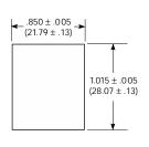
Recommended chassis thickness .039" (.99mm) to .079" (2.01mm).
