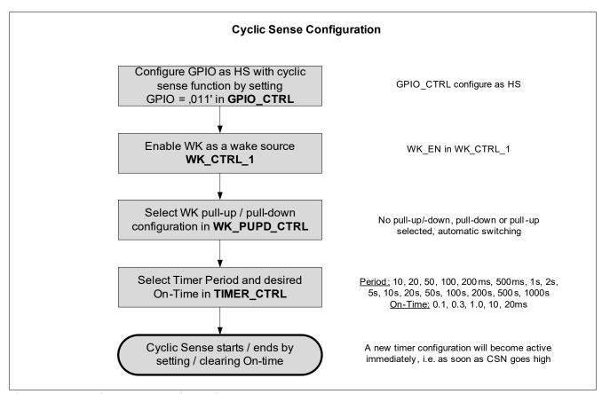
Figure 7 Cyclic Sense: Configuration and Sequence
