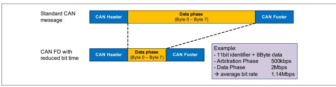
Figure 25 Bite Rate Increase with CAN FD vs. Standard CAN
