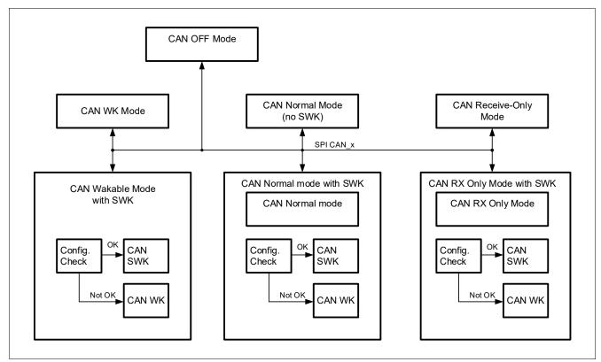
Figure 17 CAN SWK State Diagram
