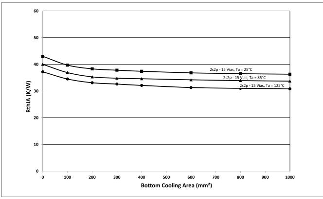
Figure 54 Thermal Resistance ( $R_{\rm th\_JA}$ ) vs. Cooling Area
