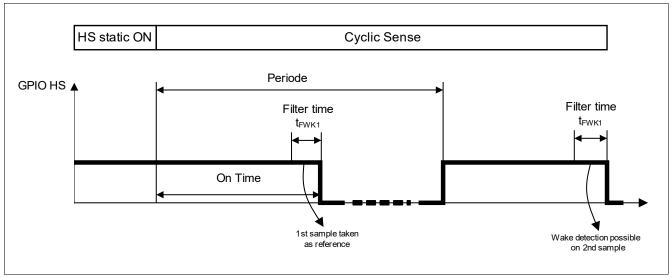
Figure 8 Cyclic Sense Timing
