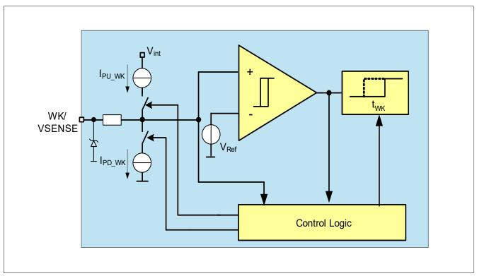
Figure 30 Wake Input Block Diagram
