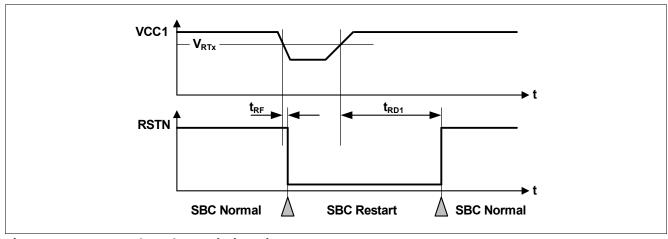
Figure 42 VCC1 Undervoltage Timing Diagram
