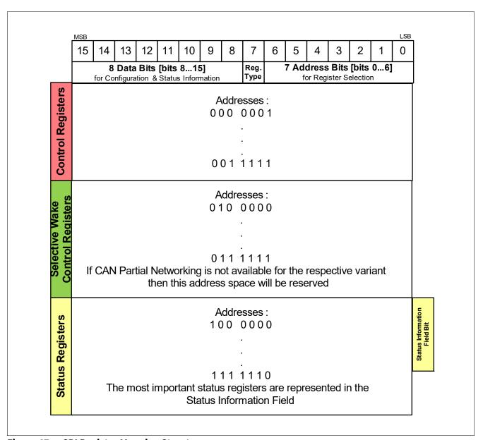
Figure 47 SPI Register Mapping Structure
