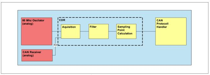
Figure 18 Clock and Data Recovery Block Diagram
