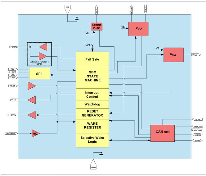
Figure 1 TLE9471-3ES V33 Block Diagram
