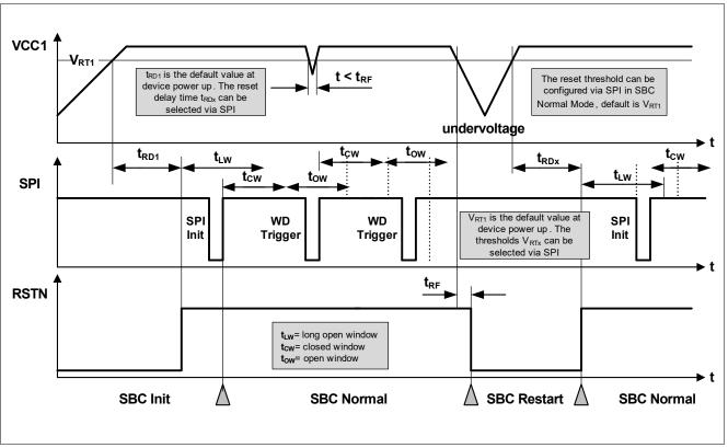
Figure 37 Reset Timing Diagram
