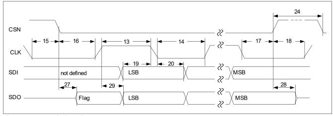
Figure 49 SPI Timing Diagram
