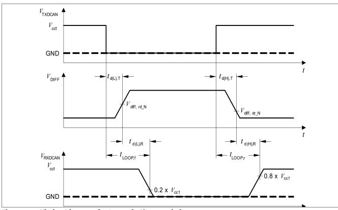
Figure 28 Timing Diagrams for Dynamic Characteristics
