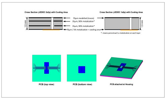
Figure 55 Board Setup
