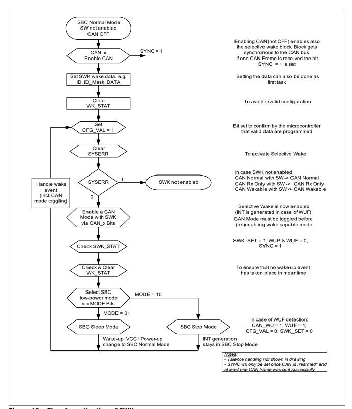
Figure 15 Flow for activation of SWK
