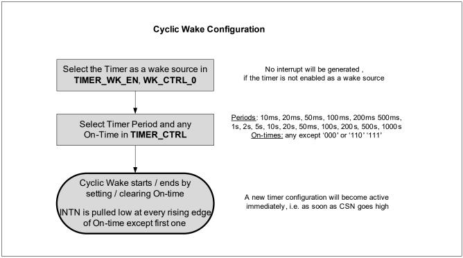
Figure 11 Cyclic Wake: Configuration and Sequence
