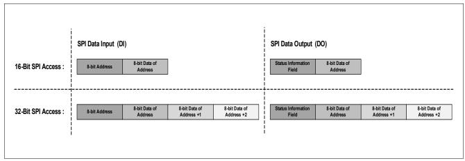
Figure 46 Data access for 16- and 32-bit SPI commands
