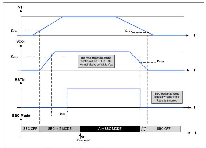
Figure 41 Ramp up / down example of Supply Voltage
