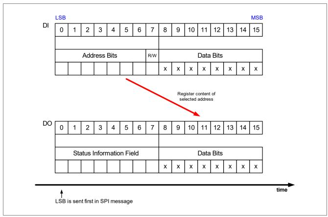
Figure 45 SPI Operation Mode
