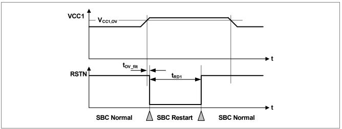
Figure 43 VCC1 Over Voltage Timing Diagram
