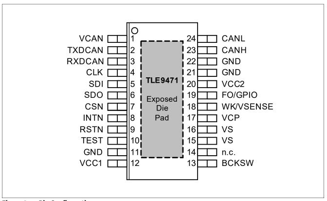
Figure 2 Pin Configuration
