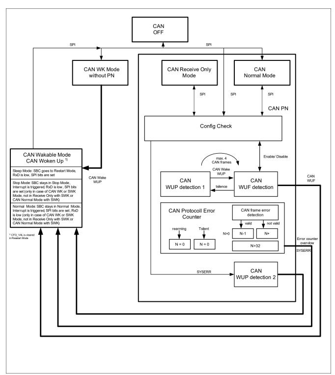
Figure 14 CAN Selective Wake State Diagram
