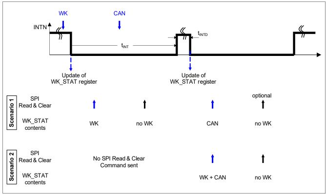
Figure 34 Interrupt Signalization Behavior
