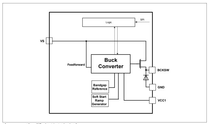
Figure 19 Simplified DC/DC Block Diagram
