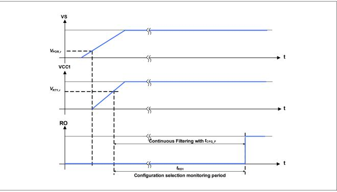
Figure 4 Hardware Configuration Selection Timing Diagram
