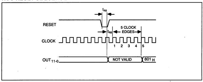
**A.C. CHARACTERISTICS** (Operating Conditions:  $V_{DD}$ = 5.0 V ± 5%,  $V_{SS}$ =0 V,  $T_a$ = 0° to 70° C (Commercial)  $V_{DD}$ = 5.0 V ± 10%,  $V_{SS}$ =0 V,  $T_a$ =-55° to 125° C (Military)
