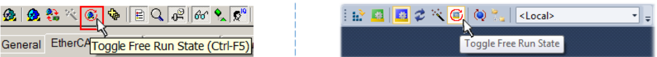
Fig. 79: TwinCAT can also be switched to this state by using a button (left: TwinCAT 2; right: TwinCAT 3)
