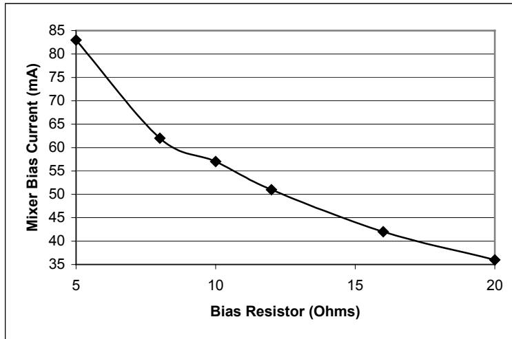
Figure 7. Mixer Bias Current vs. Bias Resistor (RA2, RB2)
