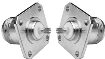
Our **in-house** machining capability now includes production of type N flange receptacles with one-piece bodies, replacing the old machined body/stamped flange method. With no unsightly solder joints, these connectors have enhanced appearance and strength compared with two-piece designs. The machined flanges are flatter than stamped flanges, and our high-speed turning centers can produce any volume required to fill your production quantity needs.
