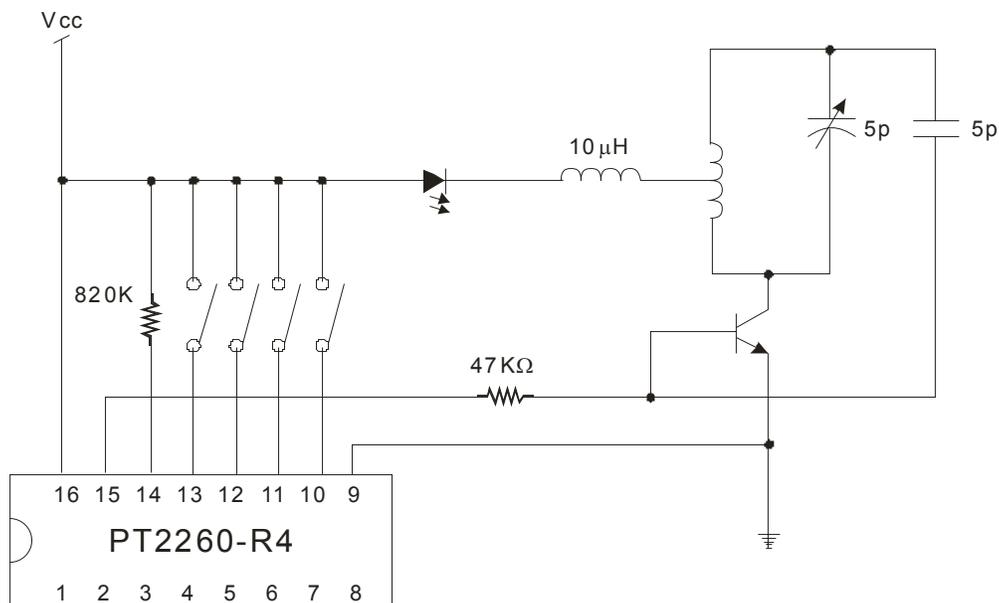
UHF Band 4-Data Transmitter Circuit is recommended.
