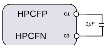
Figure 41. Charge pump flying capacitor
