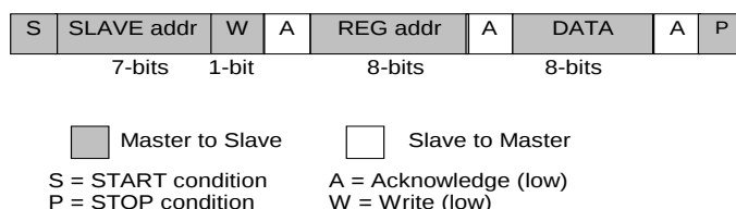
Figure 27. I 2 C byte write (SDA signal)
