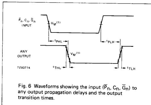
Fig. 6 Waveforms showing the input ( $\bar{P}_n, C_n, \bar{G}_n$ ) to any output propagation delays and the output transition times.
