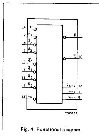
Fig. 4 Functional diagram.
