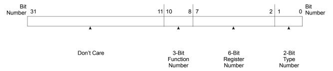
PCI-649 only responds to Type 0 configuration cycles. Type 1 cycles, which pass a configuration request on to another PCI bus, are ignored.
