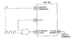
CONTINUOUS CONVERSION WITH EXTERNAL CLOCK—For continuous conversion of the input signal, the Convert Command and Clock Inhibit inputs are tied low and an external clock applied to the Clock Input. The converter will then continuously convert, reset and initiate new conversions. The converter will be reset on the 13th clock pulse, and the subsequent appropriate will be resident with a 14th clock pulse. The
