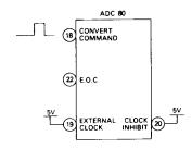
**OPERATION WITH EXTERNAL CLOCK**—The external clock is connected and gated as shown. The Convert Command input must be synchronized with the external clock signal and the Clock Inhibit input tied low, for proper operation.
