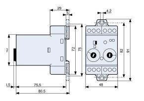
L2 plug-in casing for 11-pin socket
