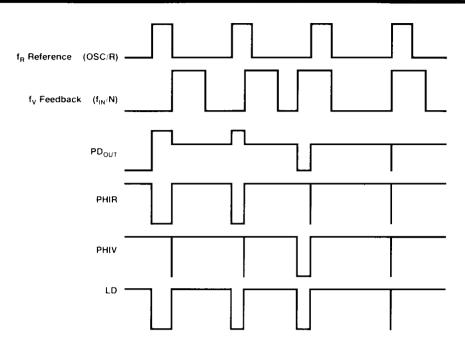
NOTE: The  $PD_{OUT}$  state is equal to either  $V_{DD}$  or  $V_{SS}$  when active. When not active, the output is high impedance and the voltage at that pin is determined by the low pass filter capacitor.
