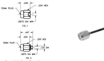
Note: Standard finish is gold plating on housing for direct solder to cable and passivated coupling nut.
