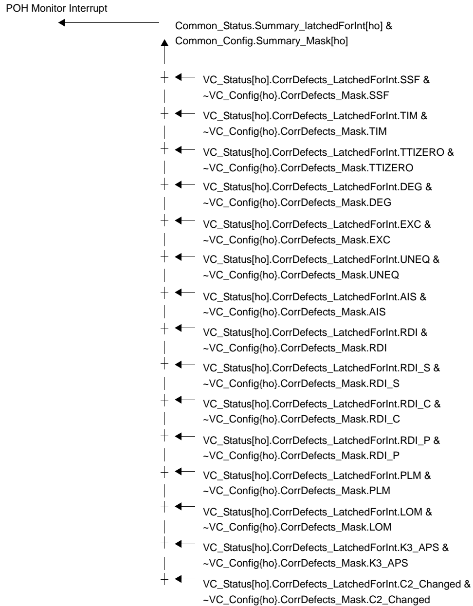
Figure 32. POH Monitor Interrupt Tree
