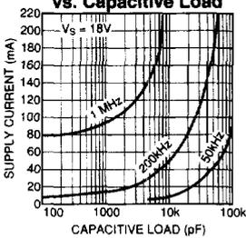
**Supply Current vs. Capacitive Load**
