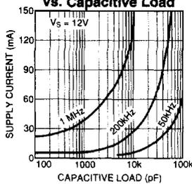
**Supply Current vs. Capacitive Load**
