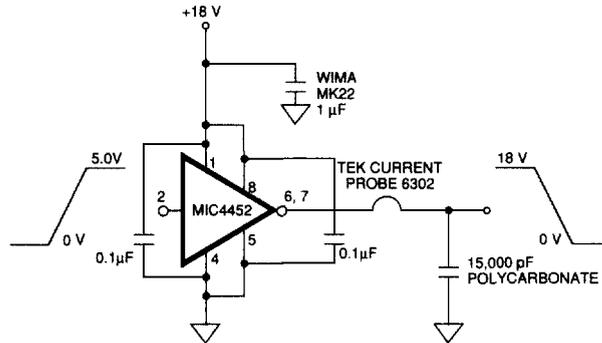
Figure 6. Peak Output Current Test Circuit
