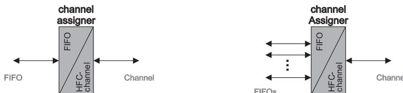
**Figure 3.7:** HFC-channel assigner in CSM
