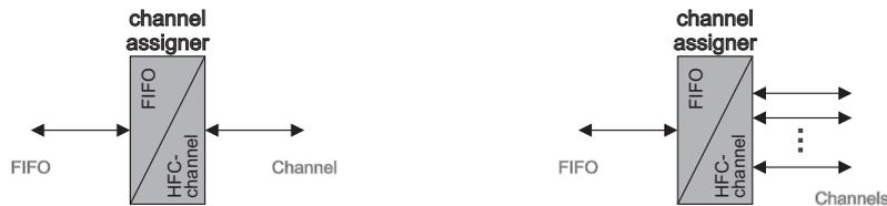
**Figure 3.9:** HFC-channel assigner in FSM
