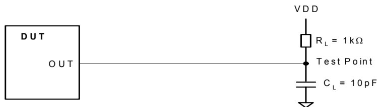
Figure 23. Load Circuit - High to Low Slew Rate Measurement
