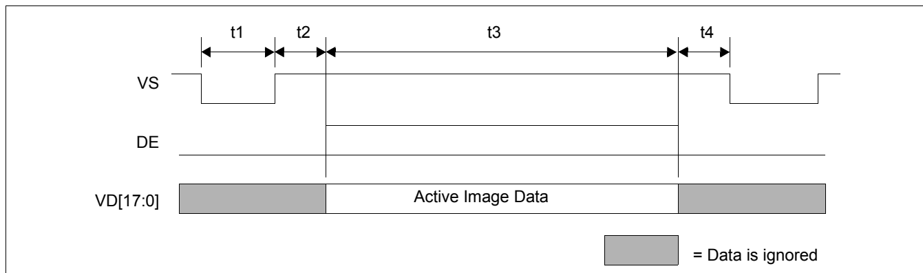
Figure 8-8: Parallel RGB Interface Vertical Timing
