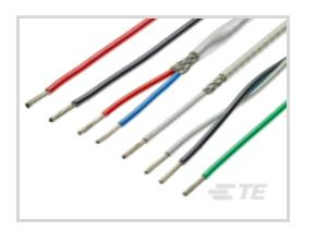
Cable Type: Spec 44 Voltage Rating: 600 VAC Insulation Material: Modified Radiation Cross-linked PVDF Conductor Material: Tin-Coated Copper Wire Size: 22 AWG
