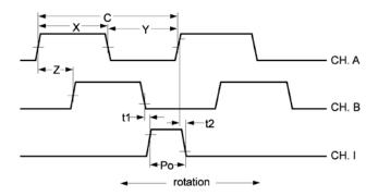
**CPR:** The number of Cycles (C) of the A or B outputs Per Revolution.
