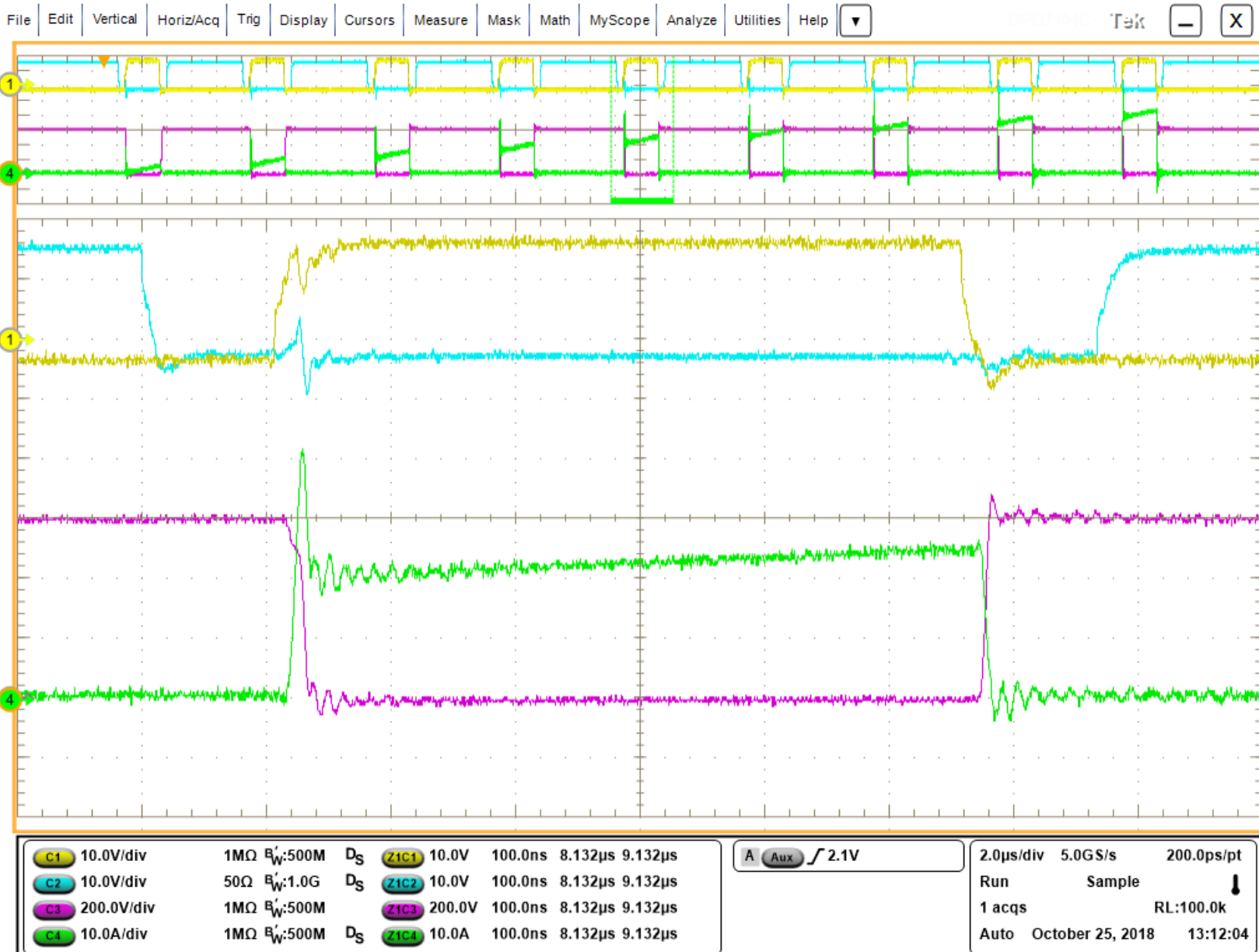
Figure 9-6. SiC MOSFET Switching Waveforms
