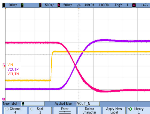
Figure 8-4. Step Response of the AMC1301-Q1
