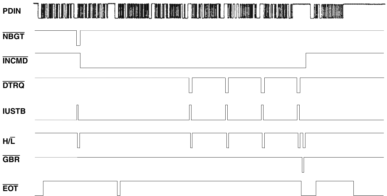
Figure 10 – RT TO RT TRANSFER OF FOUR DATA WORDS (THIS RT RECEIVING THE DATA)
