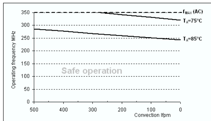
Figure 9. Maximum MPC9443 Frequency, V_{\text{CC}} = 3.3 \text{ V} , MTBF 4 Years, 4 pF Load per Line
