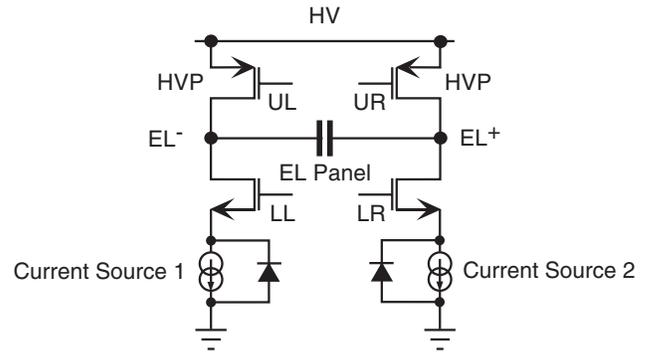
FIGURE 2: H-BRIDGE SCHEMATIC
