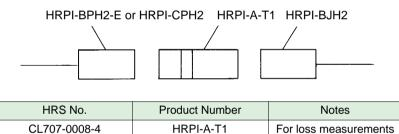
NOTE: A special terminal extraction tool, PO73-T-HPJRMV (CL350-0104-7) is required when removing HRPI-BJH2 from HRPI-A-T1.
