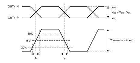
Figure 7-5. Differential Output Voltage and Rise/Fall Time
