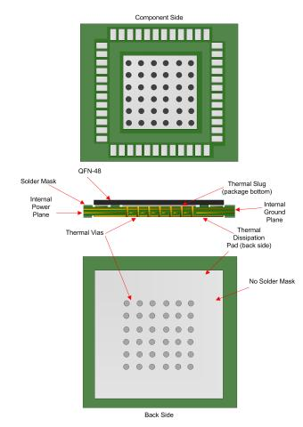
Figure 12-1. General PCB Ground Layout for Thermal Reliability (8+ Layers Recommended) - TBD
