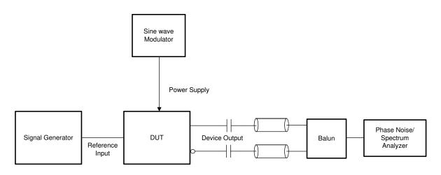
Single-sideband spur level measured in dBc with a known noise amplitude and frequency injected onto the device power supply.
