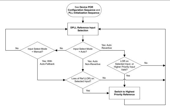
Figure 9-16. DPLL Reference Input Selection Flowchart
