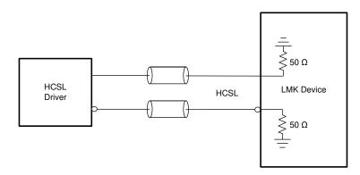
Figure 9-14. HCSL (Load Terminated) to Reference (INx)
