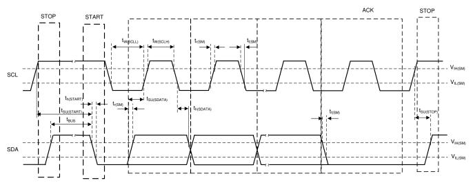
Figure 7-4. I<sup>2</sup>C Timing Diagram
