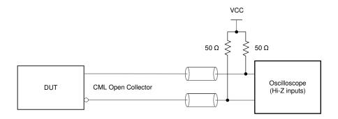
Figure 8-9. CML Open Collector Output DC Test Configuration
