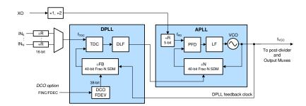
Figure 3-1. Block Diagram of Paired DPLL and APLL
