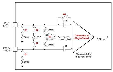
Figure 9-9. Reference Input Buffer
