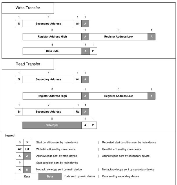
Figure 9-41. I<sup>2</sup>C Byte Write and Read Transfers
