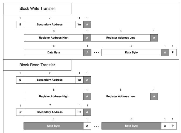
Figure 9-42. I<sup>2</sup>C Block Register Transfers
