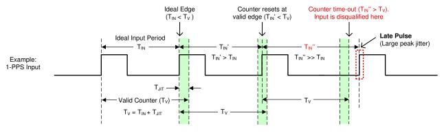
Figure 9-19. 1-PPS Input Window Detector Example
