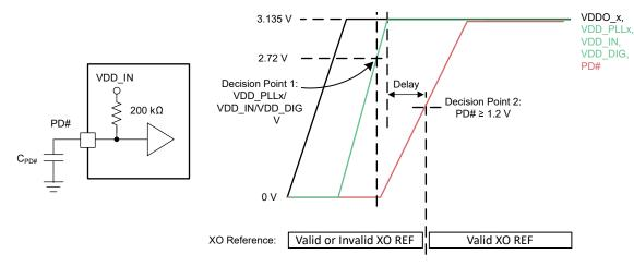
Figure 10-2. Recommendation for Power Up From Split-Supply Rails
