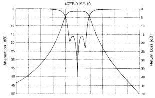
Center Frequency: 915MHz Span: 200MHz
