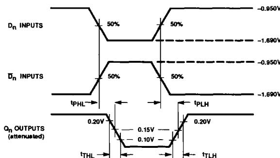
Waveform 1. Propagation Delay and Transition Times
