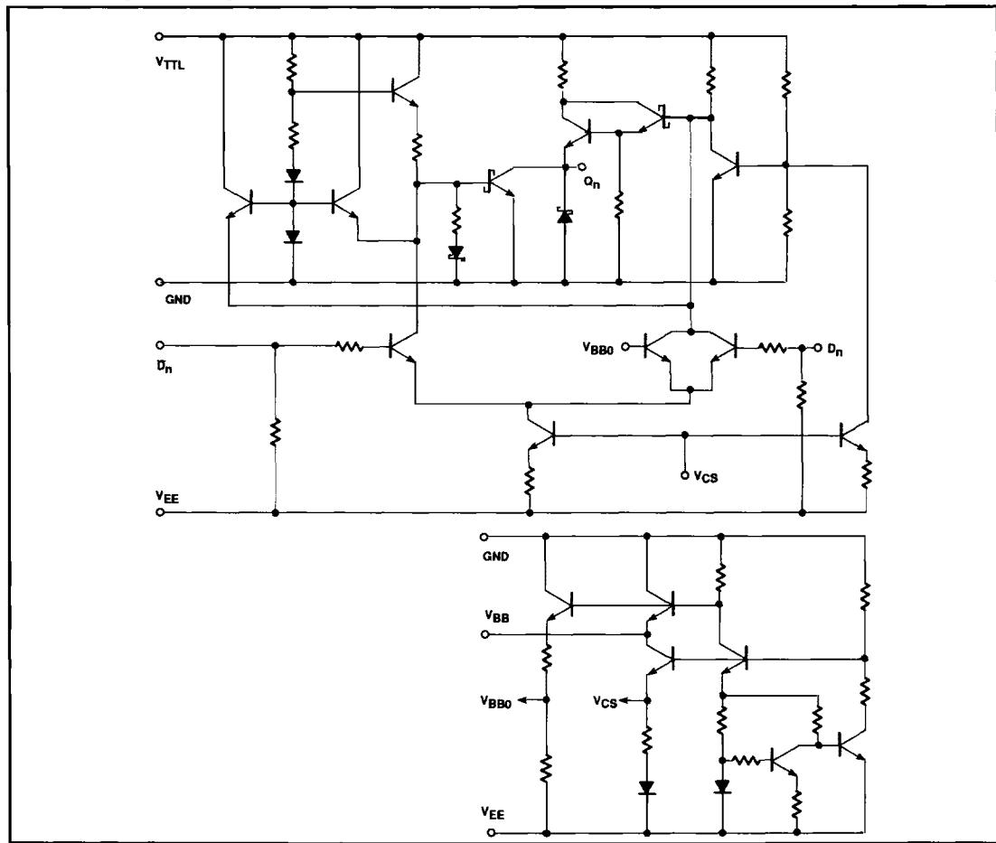
**Translator****100125****ABSOLUTE MAXIMUM RATINGS** GND = ground,  $T_A = 0^\circ\text{C}$  to  $+85^\circ\text{C}$  unless otherwise specified.
