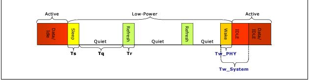
Figure 3-14. Energy Efficient Ethernet Operation
