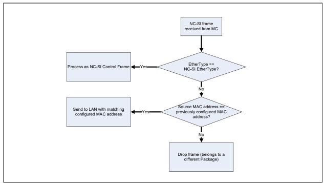
Figure 10-6. NC-SI Frames Receive Flow for the NC
