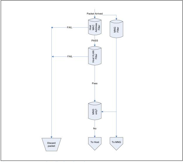
Figure 7-1. I210 Receive Filtering Flow Chart
