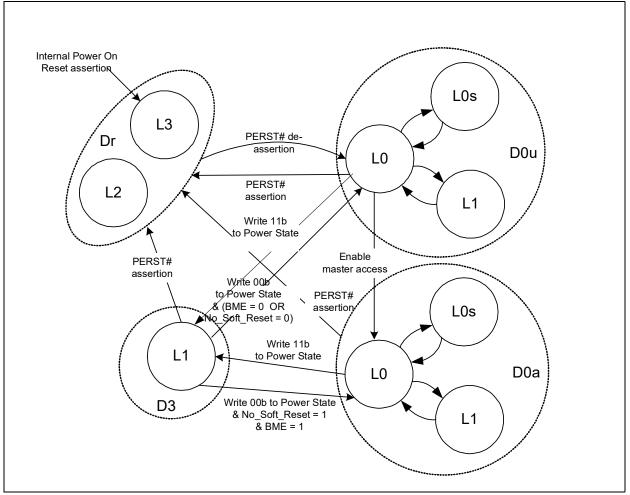
Figure 5-2. Link Power Management State Diagram
