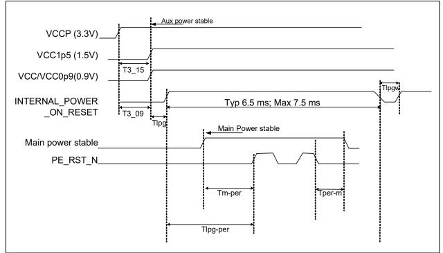
Figure 11-1. Power and Reset Sequencing
