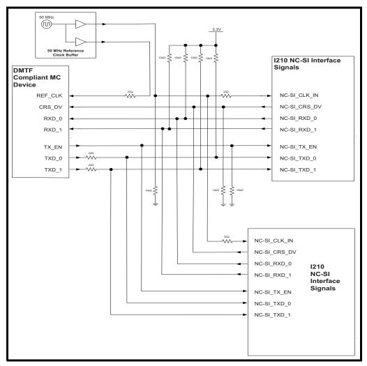
Figure 12-18.NC-SI Connection Requirements - Multi-Drop Configuration
