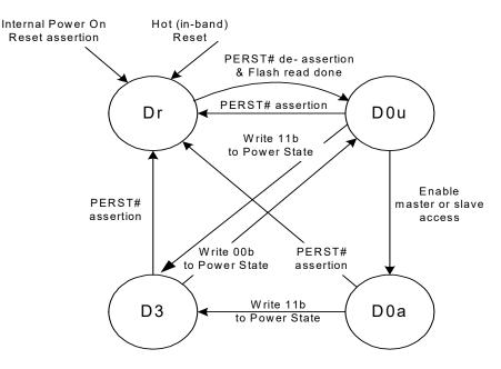
Figure 5-1. Power Management State Diagram
