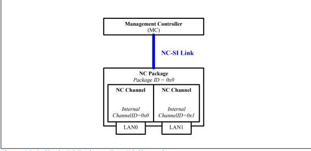
Figure 10-4. Single NC Package, Two NC Channels
