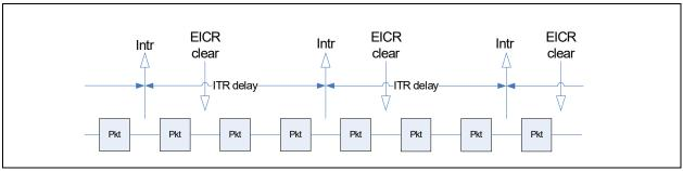
Figure 7-16. Case A: Heavy Load, Interrupts Moderated
