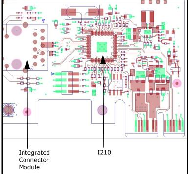
Figure 12-14.Layout for Discrete Magnetics
