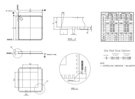
Figure 2-2. I210 QFN 9 x 9 mm Package
