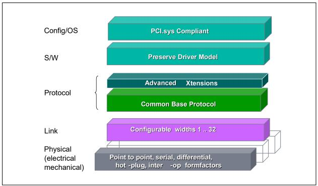
Figure 3-1. PCIe Stack Structure
