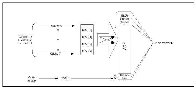
Figure 7-13. Cause Mapping in Legacy Mode
