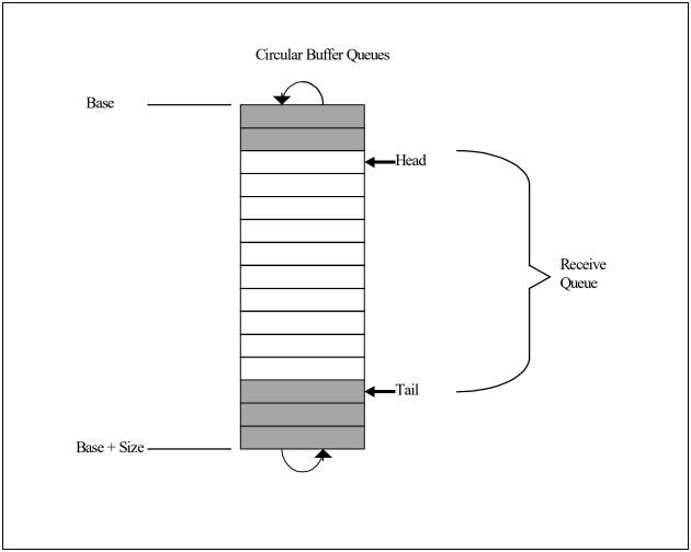
Figure 7-7. Receive Descriptor Ring Structure
