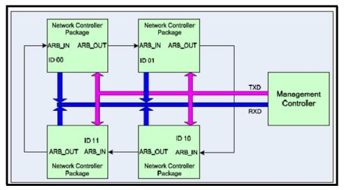
Figure 12-19.NC-SI Connection Requirements - Hardware Arbitration
