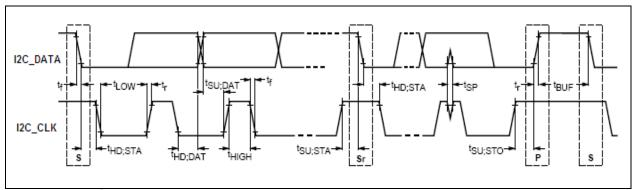
Figure 11-3. I<sup>2</sup>C I/F Timing Diagram
