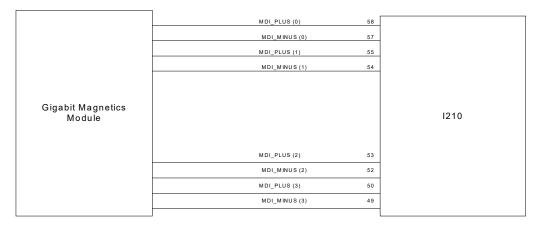
Figure 12-11.I210 Gigabit Magnetics Module Connections
