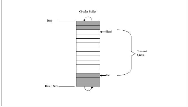
Figure 7-10. Transmit Descriptor Ring Structure
