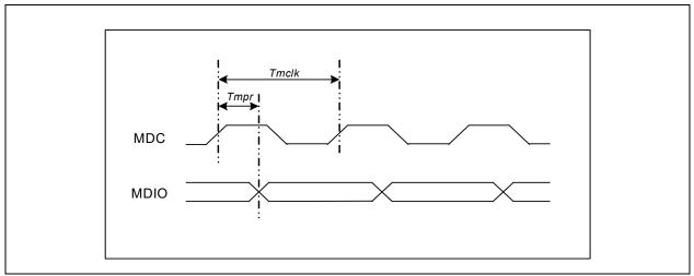
Figure 11-8. MDIO Output AC Timing Diagram
