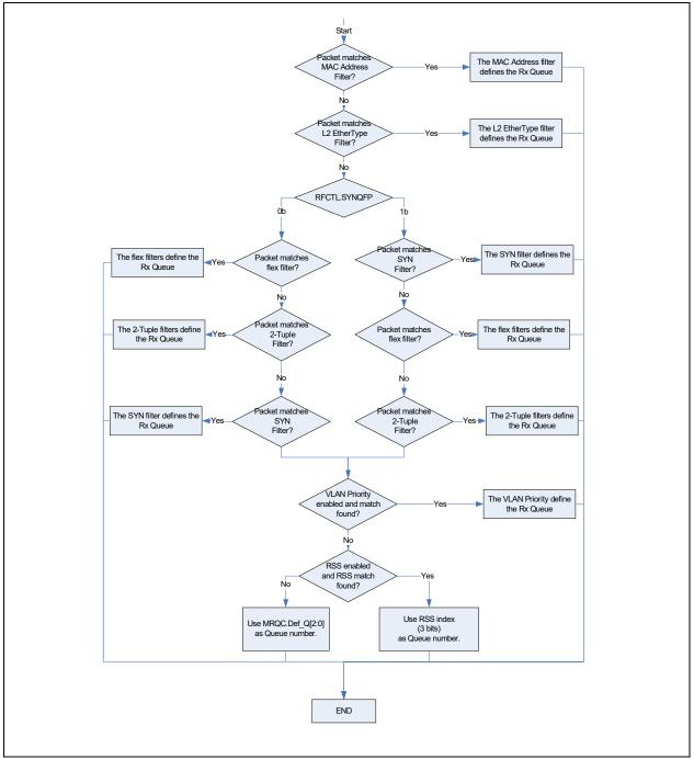
Figure 7-5. Receive Queuing Flow
