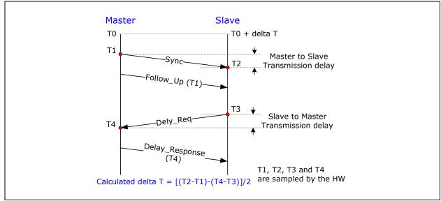
Figure 7-20. Sync Flow and Offset Calculation
