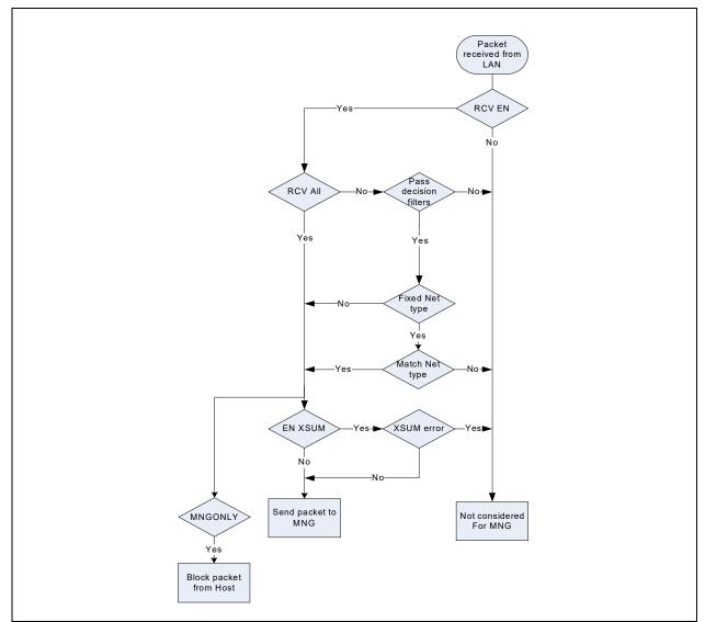
Figure 7-4. Manageability Filtering
