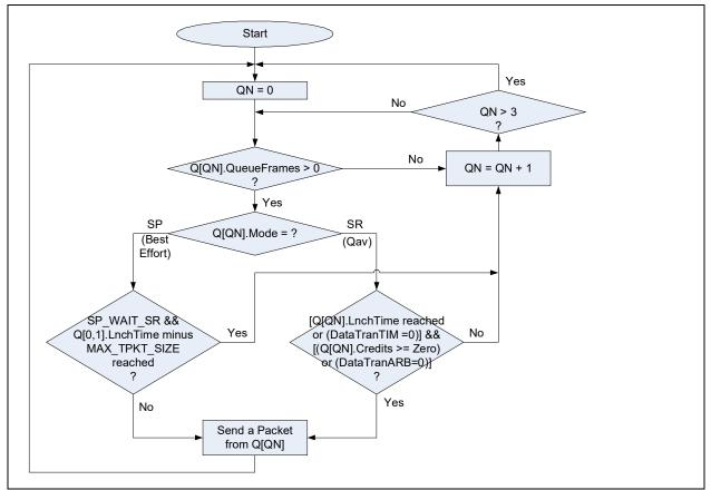
Figure 7-12. Data Transmission Arbitration Operation for TransmitMode = Qav
