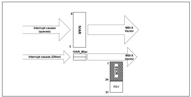
Figure 7-14. Cause Mapping in MSI-X Mode
