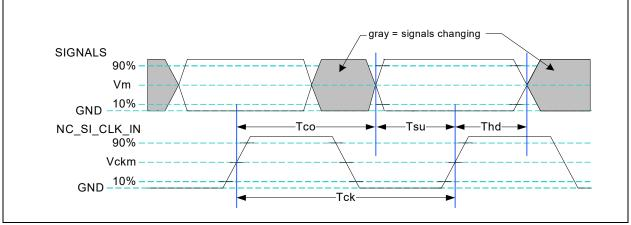
Figure 11-5. NC-SI Timing Diagram
