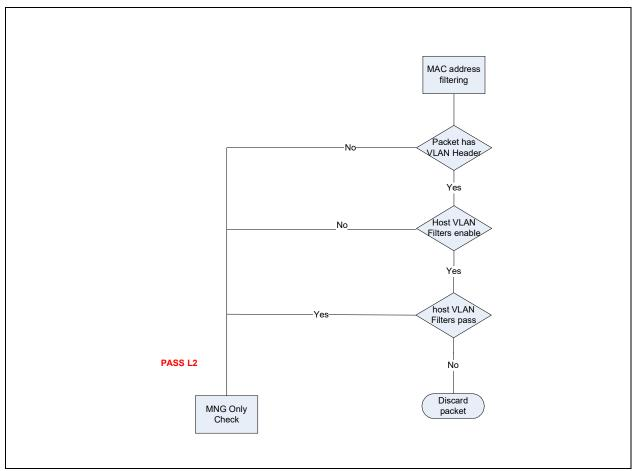
Figure 7-3. I210 VLAN Filtering
