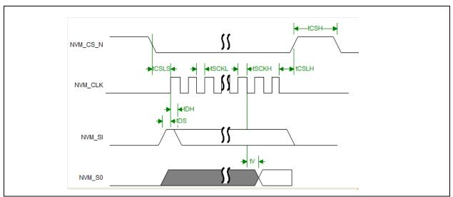
Figure 11-4. Flash Timing Diagram
