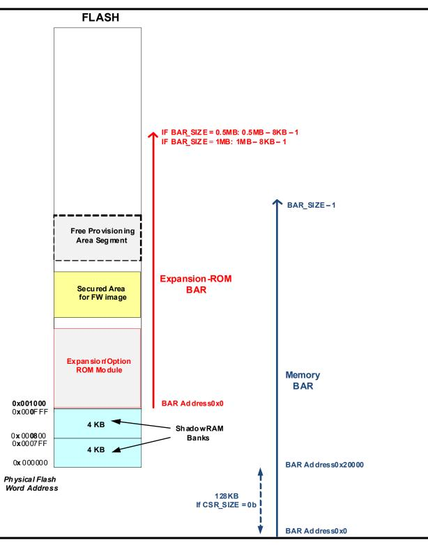
Figure 3-4. Flash Part Size is Larger Than BAR Size
