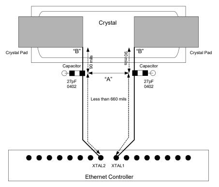
Figure 12-10.Recommended Crystal Placement and Layout
