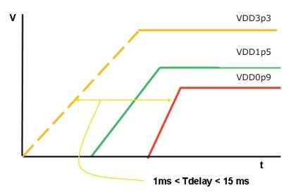
Figure 12-25.Internal SVR Power-Up Sequence
