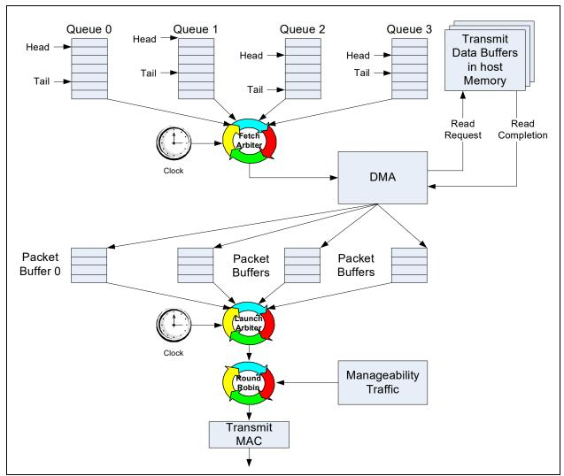
Figure 7-11. Transmit Architecture Qav Mode
