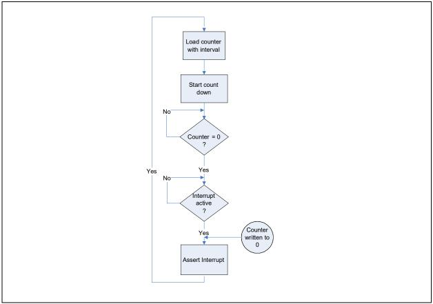
Figure 7-15. Interrupt Throttle Flow Diagram
