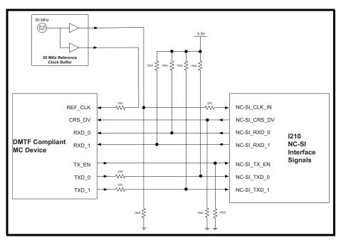
Figure 12-17.NC-SI Connection Requirements - Single-Drop Configuration
