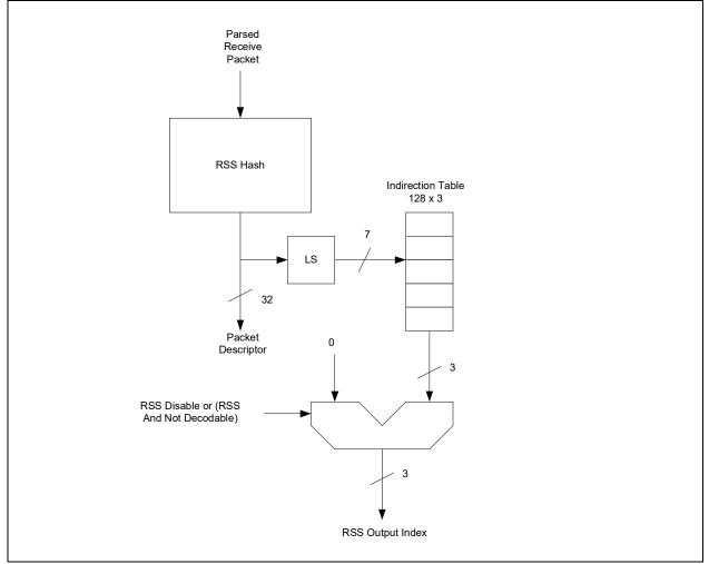
Figure 7-6. RSS Block Diagram
