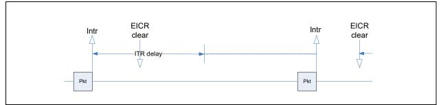
Figure 7-17. Light load, Interrupts Immediately on Packet Receive
