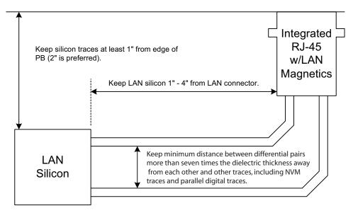
**Note:** Figure 12-13 represents a 10/100 diagram. Use the same design considerations for the two differential pairs not shown for gigabit implementations.
