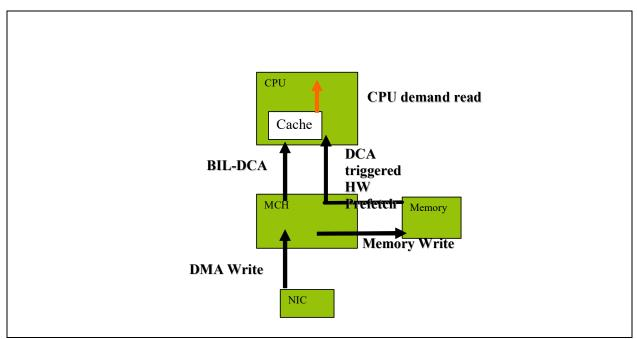
Figure 7-18. Diagram of DCA Implementation on FSB System
