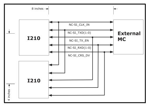
Figure 12-21.NC-SI Trace Length Requirement for Multi-Drop
