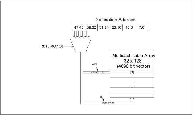
Figure 8-1. Multicast Table Array
