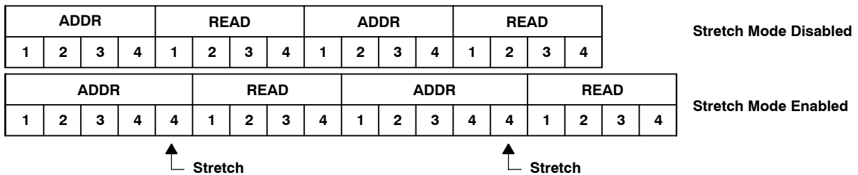
Figure 5. Two 32-Bit Nonpage-Mode Reads
