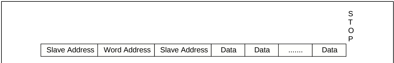
Figure 40. Serial Byte Access- Sequential Read
