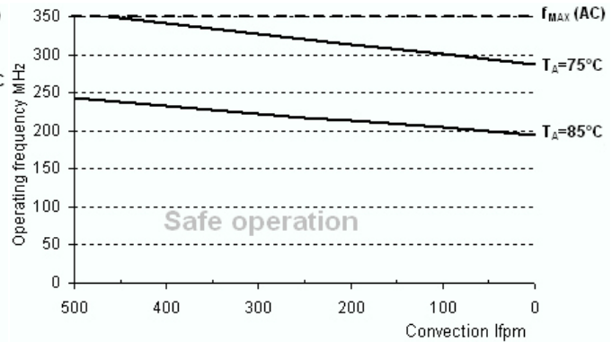
Figure 8. Maximum MPC9448 frequency, V_{CC} = 3.3V , MTBF 9.1 years, 4 pF load per line, 2s2p board
