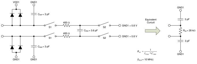
Figure 33. Equivalent Input Circuit
