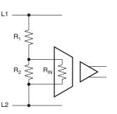
Figure 34. Voltage Measurement Application
