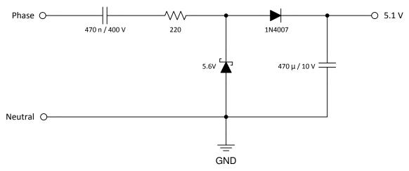
Figure 39. Cap-Drop High-Side Power Supply for the AMC1100
