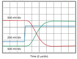
Figure 37. Typical Step Response of the AMC1100
