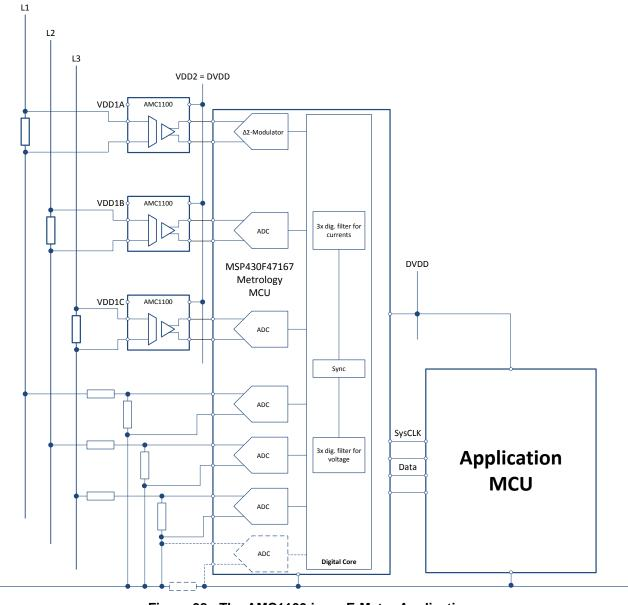
Figure 38. The AMC1100 in an E-Meter Application
