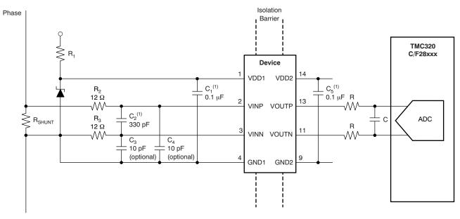
Figure 36. Shunt-Based Current Sensing with the AMC1100
