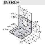
3027162 Mounting bracket, rectangular, stainless steel, for sensors with 30 mm thread, wide holes for accurate alignment
